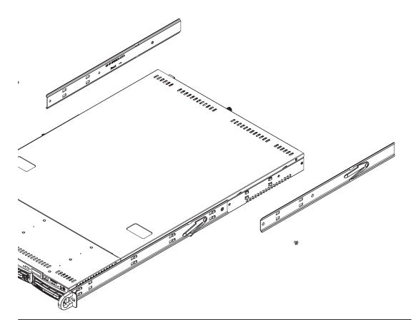
Figure 2-2. Installing the Rack Rails
